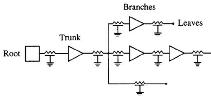
**Figure 2.6: Buffered clock tree [FRI-00].**
