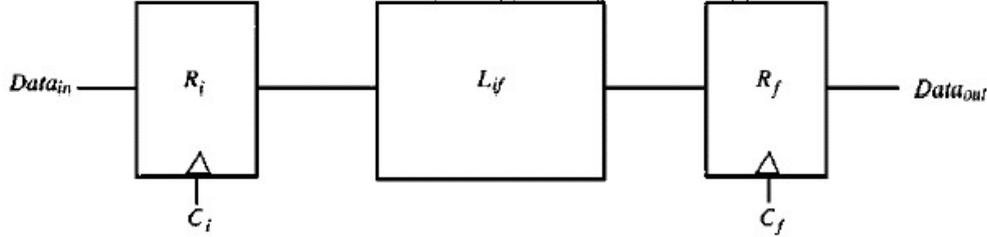
**Figure 2.1: Local data path components [FRI-00].**
