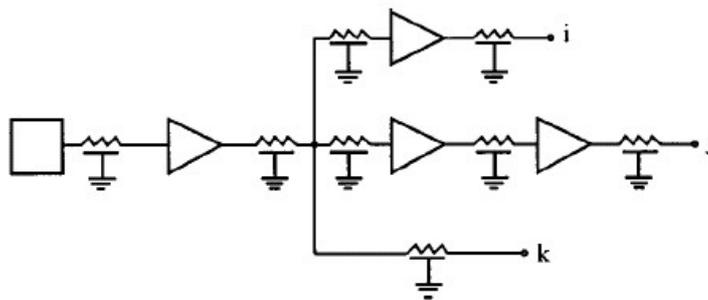
**Figure 2.12: Different interconnect impedances and capacitive loads [FRI-00].**
