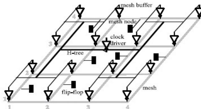
Figure 2.10: 3D view of a mesh structure [YEH-06].
