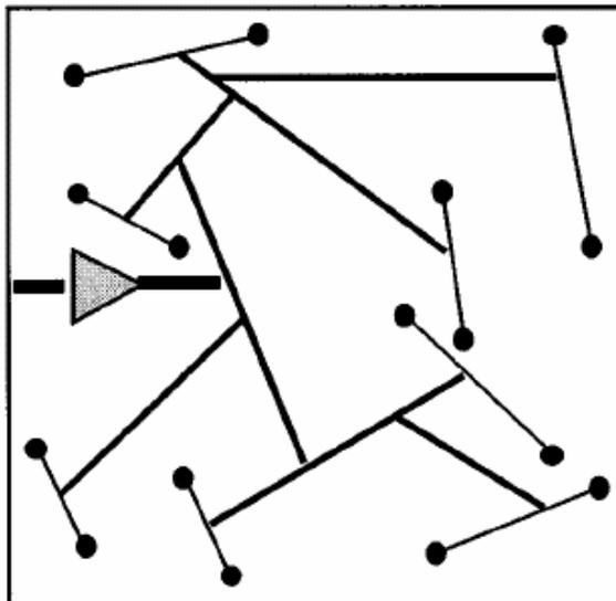
**Figure 2.7: Geometric matching for zero clock skew [FRI-00].**
