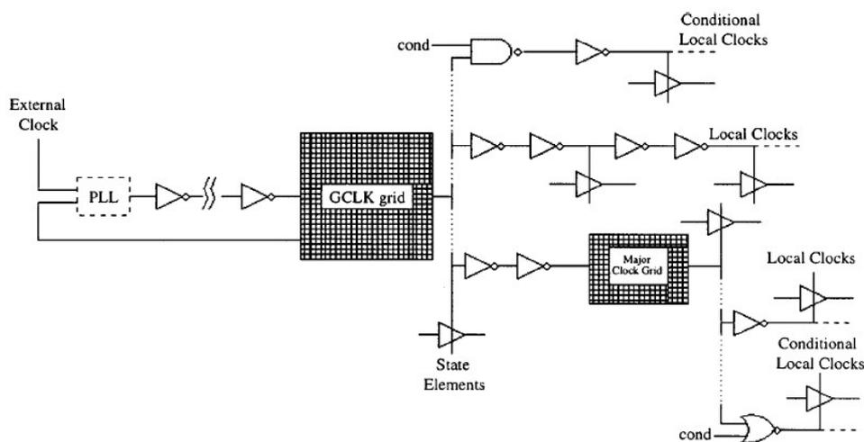
**Figure 2.18: Hierarchy in Alpha 21264 microprocessor clock network [GRO-98].**
