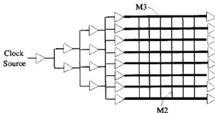
**Figure 2.17: Clock distribution network of Alpha 21064 microprocessor [HOR-92].**
