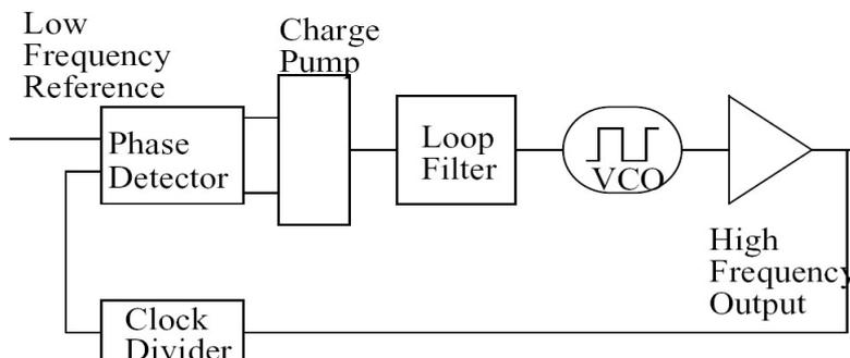
**Figure 2.5: Generic PLL block diagram [STE-97].**
