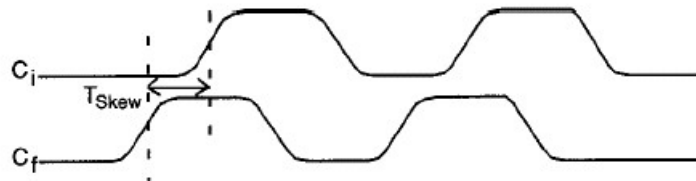
Figure 3.1: Positive clock skew.
