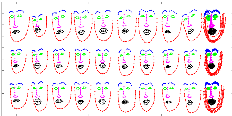
Figure 4.7: First frame of a sequence for 9 Spectrum subjects. Top: Zero centered faces of the original sequences. Middle: Similarity aligned using most rigid points (nose, eye corners). Bottom: Affine aligned using most rigid points. Right: Superimposed shapes.
