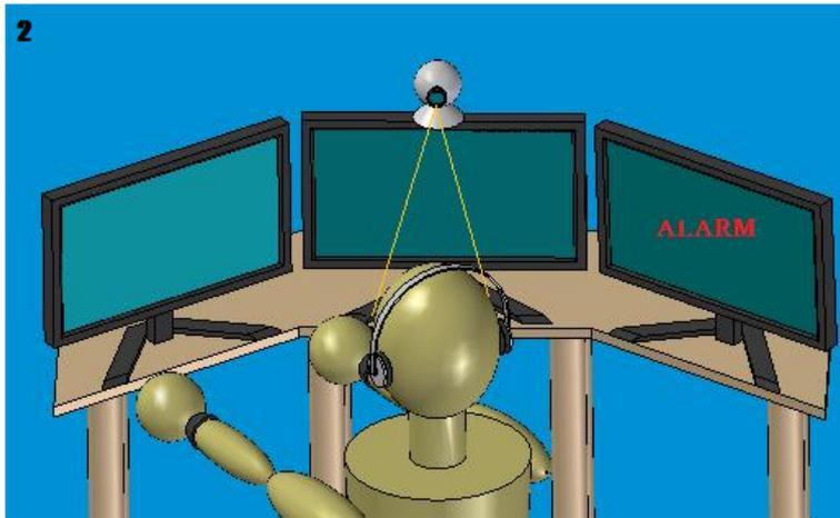
Figure 4.3: Head-Tracking system detects the position of the operator's head
