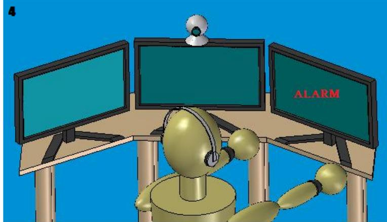
Figure 4.5: Operator is looking at right screen so alarm in the other screen disappears
