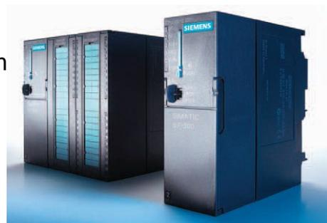
Fig 1.4: CPU S7 – Siemens
