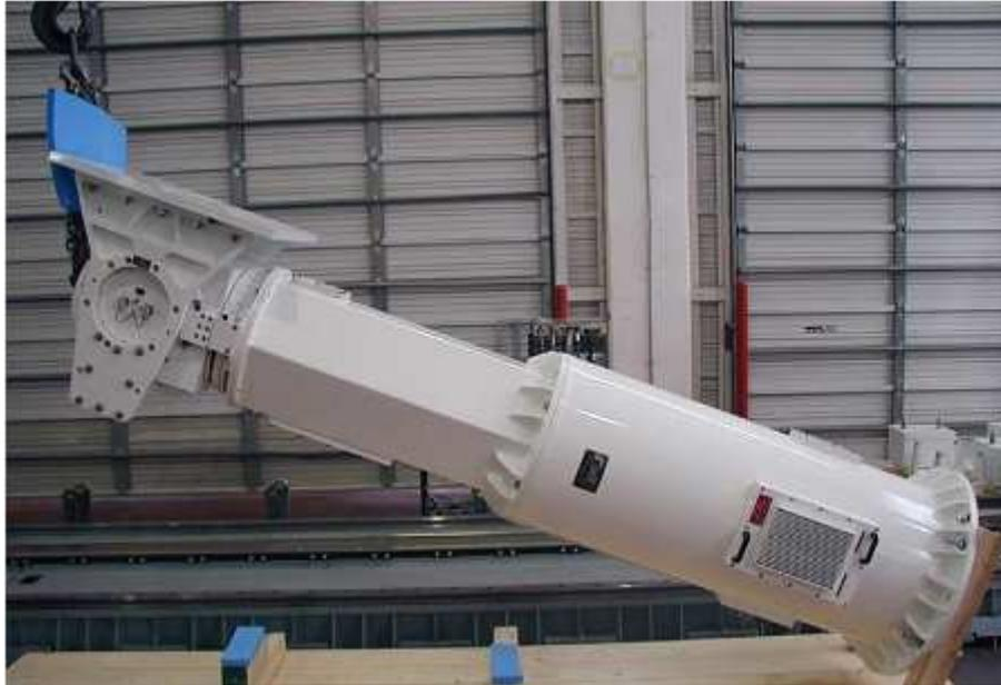
**Figura 3: AL-4018-1 Elevation over Azimuth Antenna Positioner [5]**
