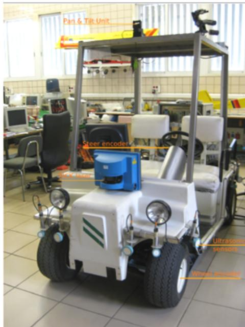
Figura 2.5: Robot Romeo-4R. Sensores (II).
