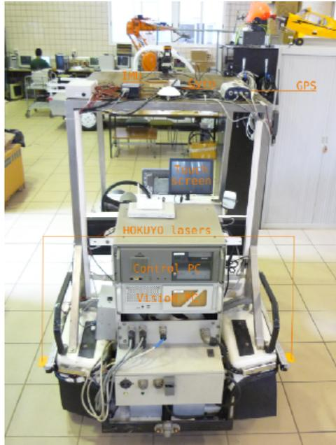
Figura 2.4: Robot Romeo-4R. Sensores (I).
