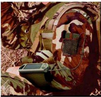
Fig. 10: Medis/General Dynamics fuel cell PDA.
