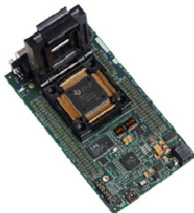
*Figura 6.4. eZdsp F28335 Starter Kit de Spectrum Digital Inc.*
