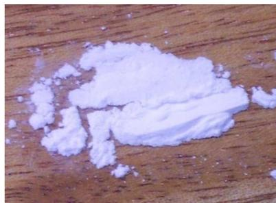
*Figura 15 Microencapsulated PCM commercialised by BASF [17].*
