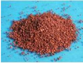
*Figura 9. Rubitherm granulate GR 41, 1 – 3 mm [58].*
