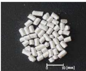
**Figura 13. Granulated PCM [122].**
