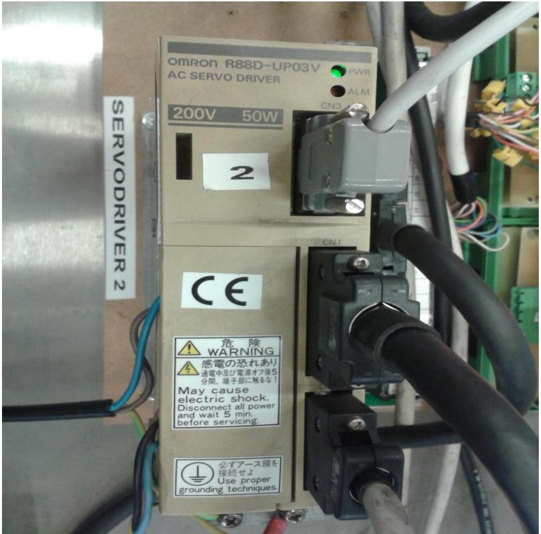
Figura 2 – 18 Servo Driver R88D-UP03V
