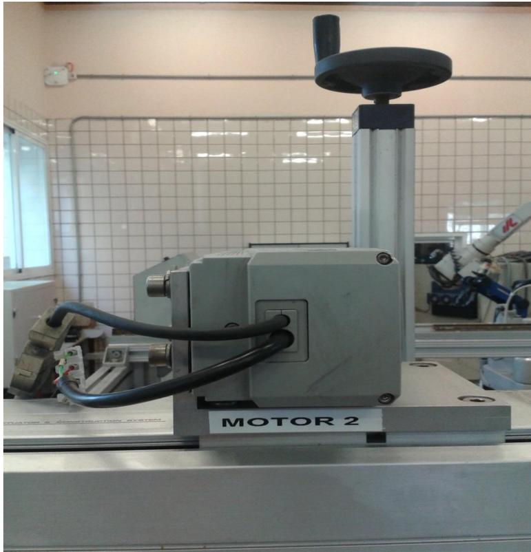
Figura 2 – 19 Servo Motor Driver R88M-U05030VA-S1
