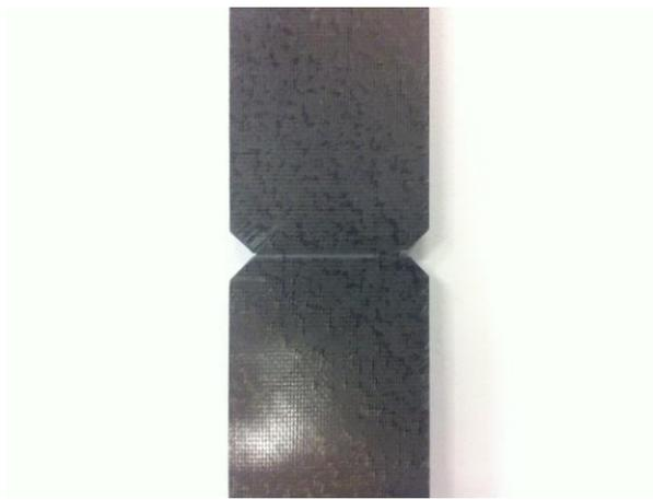
**Figura 3-30.** *Probeta DENT.*
