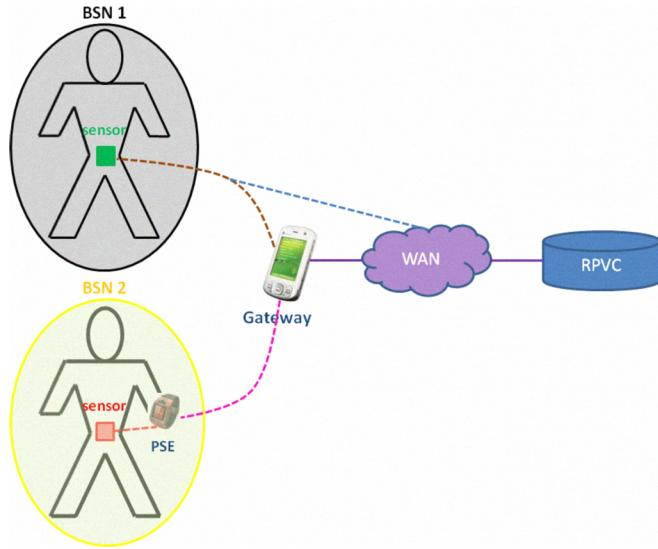
Fig. 1. Block Diagram of the two Scenarios: Single Sensor Scenario (BSN1) and Distributed Processing Scenario (BSN2).
