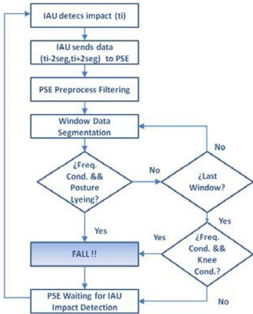
Fig. 5. Algorithm flow diagram. Freq. Cond.: frequency condition; Knee Cond.: knee fall condition.
