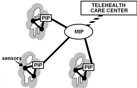
Fig. 1. Scheme of the proposed Multidevice Personal Intelligent Platform.
