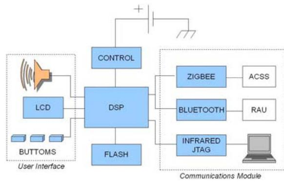
Fig. 2. Block diagram of the PSE hardware architecture.
