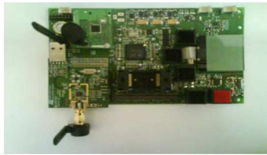
Fig. 6. PSE hardware prototype.
