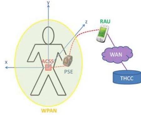
Fig. 1. Portable monitor architecture. ACSS: accelerometer smart sensor; PSE: personal server; RAU: remote access unit; WAN: wide area network; THCC: telehealthcare center.
