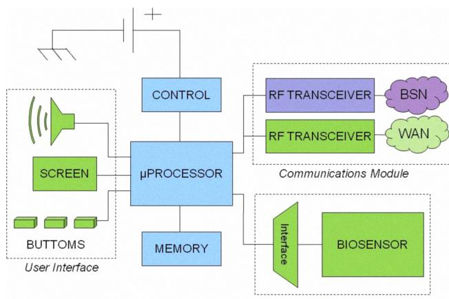
Fig. 2. Block diagram of the Smart Device hardware architecture. Green color represents modules that do not appear in every Smart Device.
