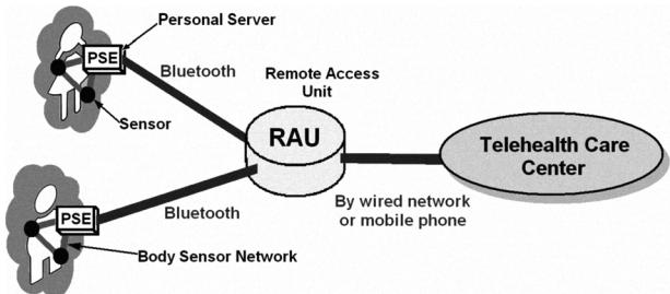
Fig. 1. Block diagram of the proposed distributed monitoring system.
