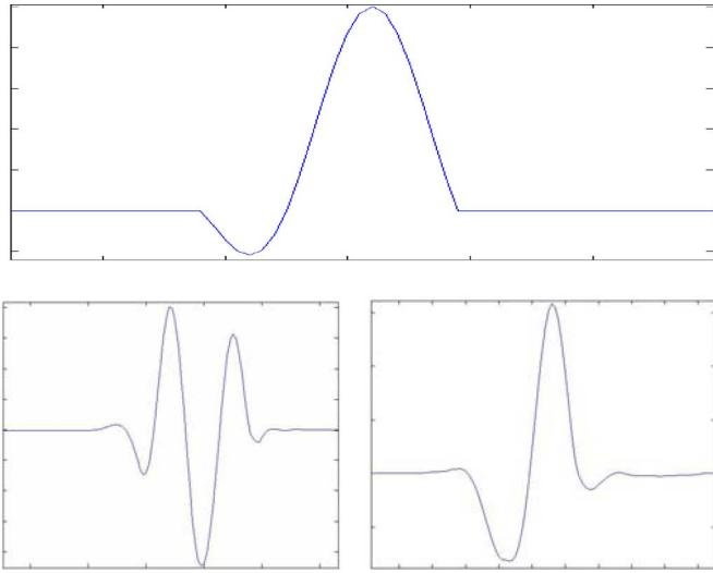
Fig. 4. (Top) Built waveform and its convolution with the vertical component of (bottom, left) knee fall and (bottom, right) vertical jump (horizontal axis in number of samples at 40 Hz for the 4-s window, vertical axis in integer dynamic range ACSS units [32]).
