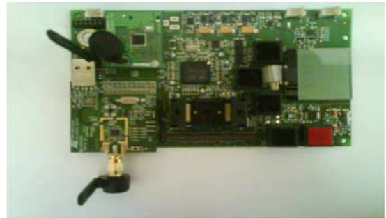
Fig. 6. PSE hardware prototype.
