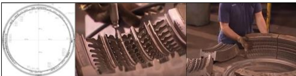
Figure 5: Drawing of a mold and sectors of a mold for tire manufacturing
