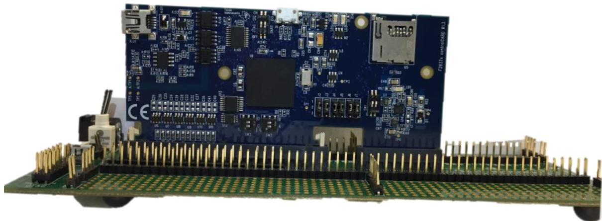
Figura 22. Conjunto de ControlCard Docking Station R4.1 con F2837x ControlCard R1.3
