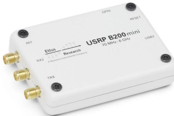
Figura 2.5 USRP Bus Series, modelo B200 mini.
