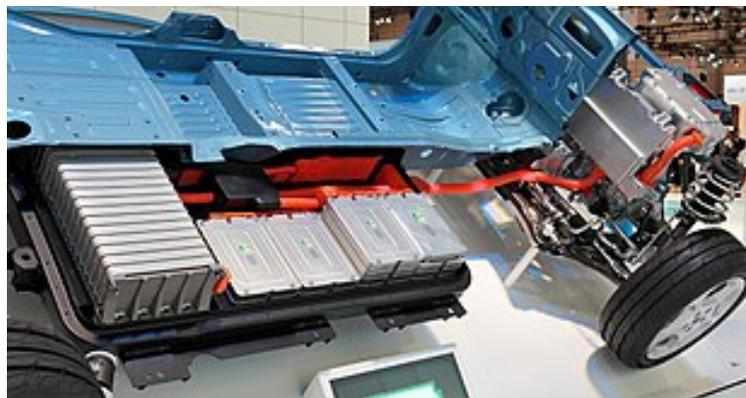
**Figura 1.9** Batería Li-ion implementada en Nissan Leaf. Fuente: [https://en.wikipedia.org/wiki/Electric\\_vehicle\\_battery](https://en.wikipedia.org/wiki/Electric_vehicle_battery).
