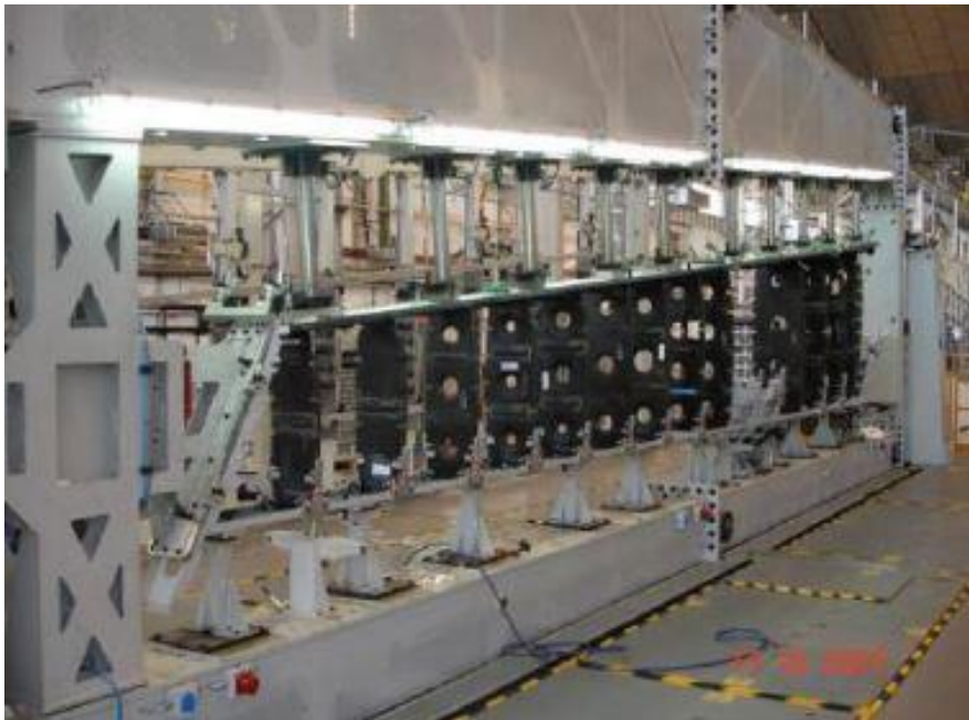
Figure 37. A400M HTP assembly (courtesy by Benasuly [17]).
