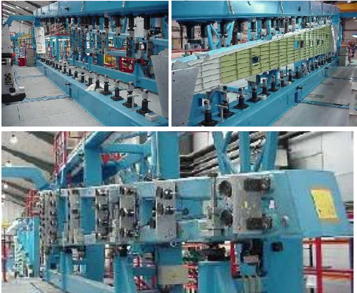
Figure 41. Stage 1 tooling station main frame (upper left), mounted bottom panel (upper right) and blades detail (down) (courtesy by Benasuly [17]).
