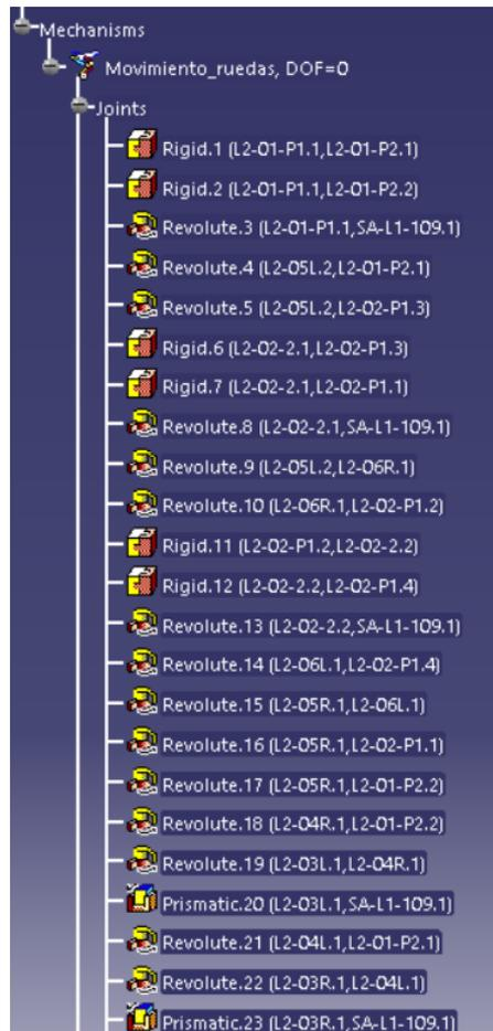
Figura 6-1 Arbol de DMU Kinematics Parte 1
