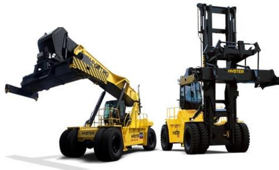
Fig. 10. Reach Stacker vs Front Lift Truck
