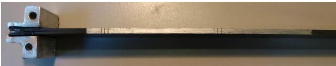
Figura 33 – Probeta AITM 10053
