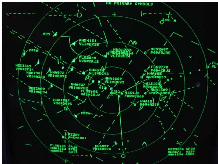
Figura 3.3. Imagen radar ATC
