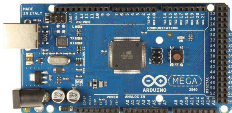
Figura 11: Arduino Mega 2560
