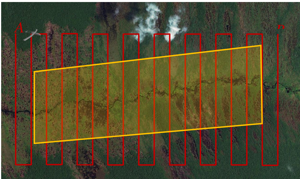
Fig. 61 Flight plan over Sabangau River (Borneo) 2494.3 m x 1196 m (298.3 Ha) [ESA's Sentinel-2] Scale 1:9000
