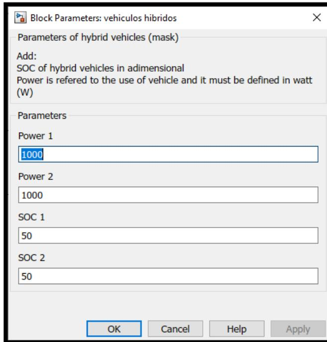
Figure 32. The general mask of hybrid vehicle
