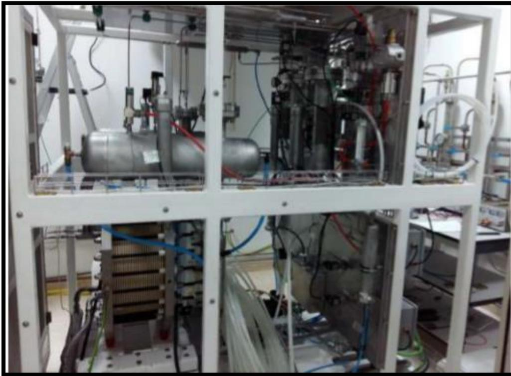
Figure 9. Electrolyser
