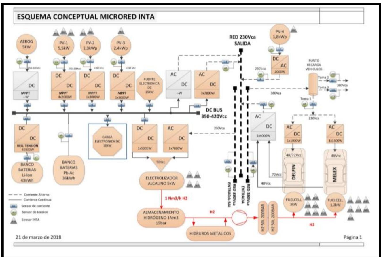
Figure 2. Scheme of INTA microgrid
