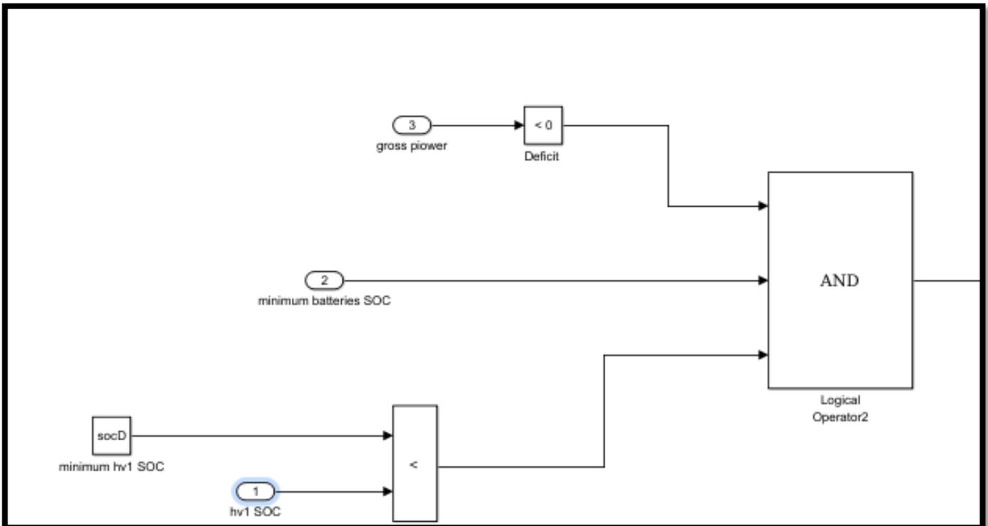
Figure 54. Scheme of discharging HV1
