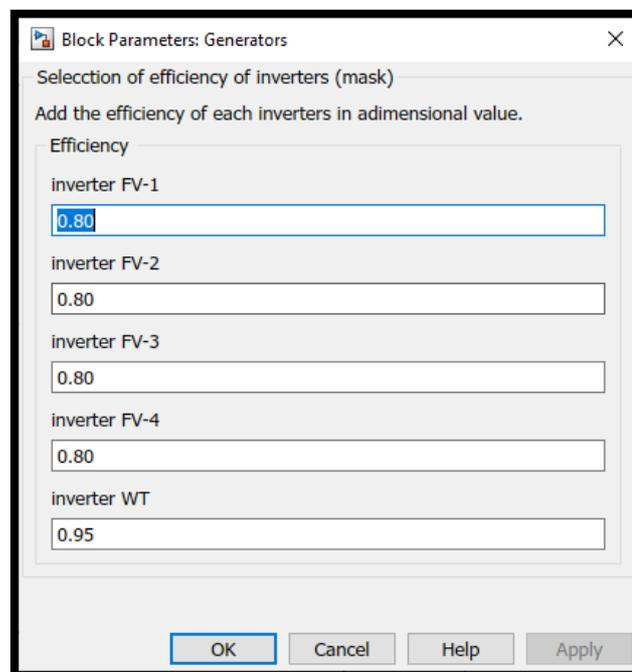
Figure 12. Mask of inverters for generators
