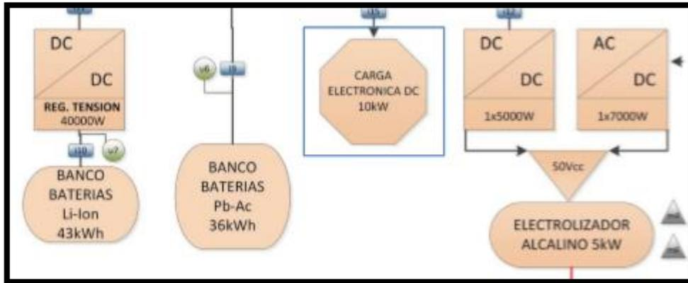
Figure 5. Scheme of SES (LB-LhB-Electrolyzer)
