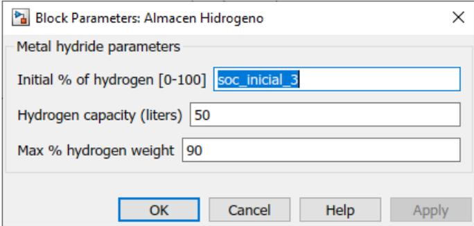
Figure 30. Mask of hydrogen storage
