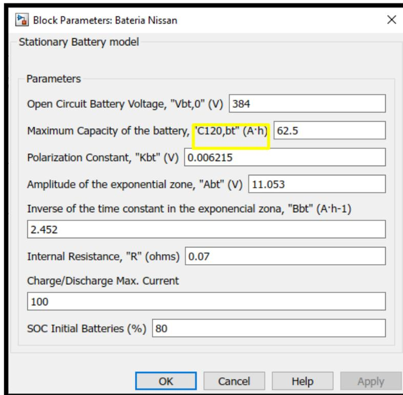
Figure 21. Mask of battery
