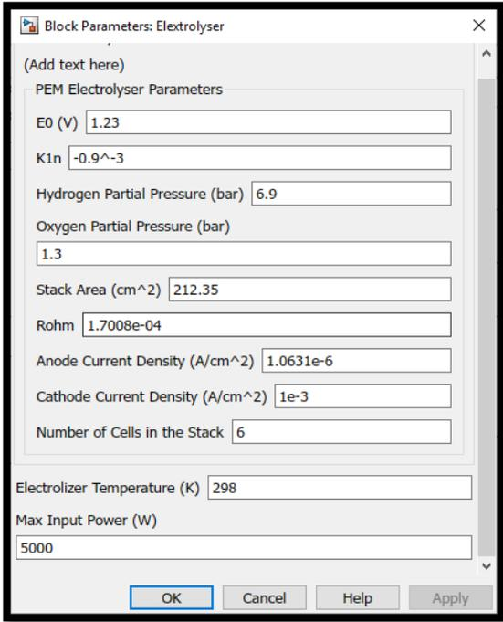
Figure 29. Mask of electrolyser
