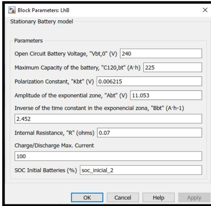
Figure 28. Mask of Lhb' battery
