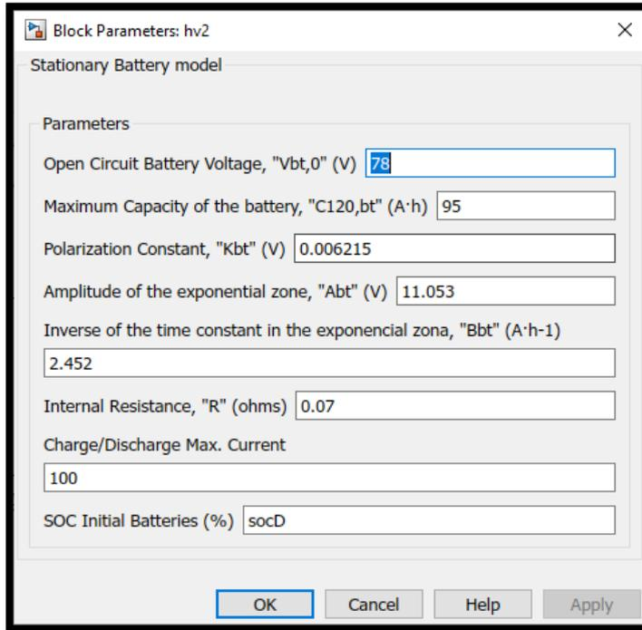
Figure 36. Mask of technical data of hv2
