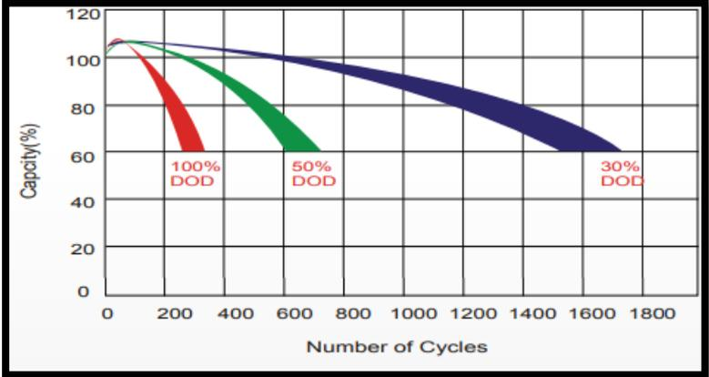
Figure 57. SOC vs Cycle (depending on DoD)
