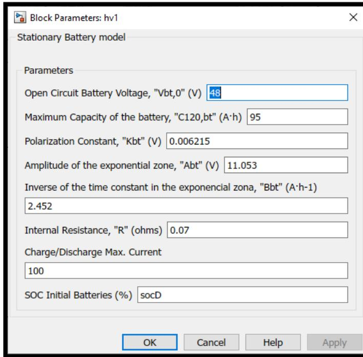
Figure 34. Mask of technical data of vh1
