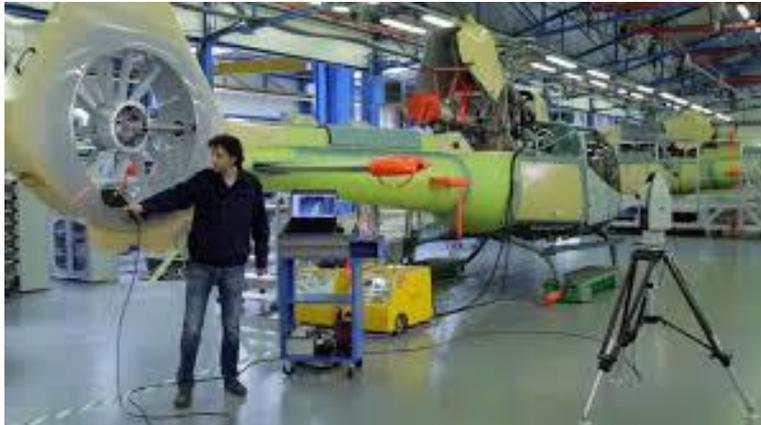
Figura 2.2 Leica Absolute Tracker AT960 de Hexagon en Airbus Helicopters [14]
