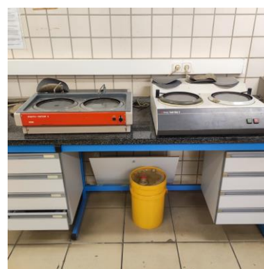
Figura 3.10 Esmerilladora Knuth-Rotor 2 y 3 de Struers.
