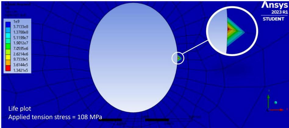
Figure 33: Fatigue Tool Life plot. Zoom of the circular notch
