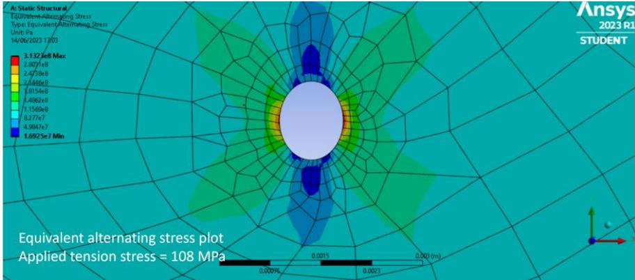
Figure 37: Fatigue Tool Equivalent Alternating Stress plot (equivalent of von Mises). Zoom of the circular notch
