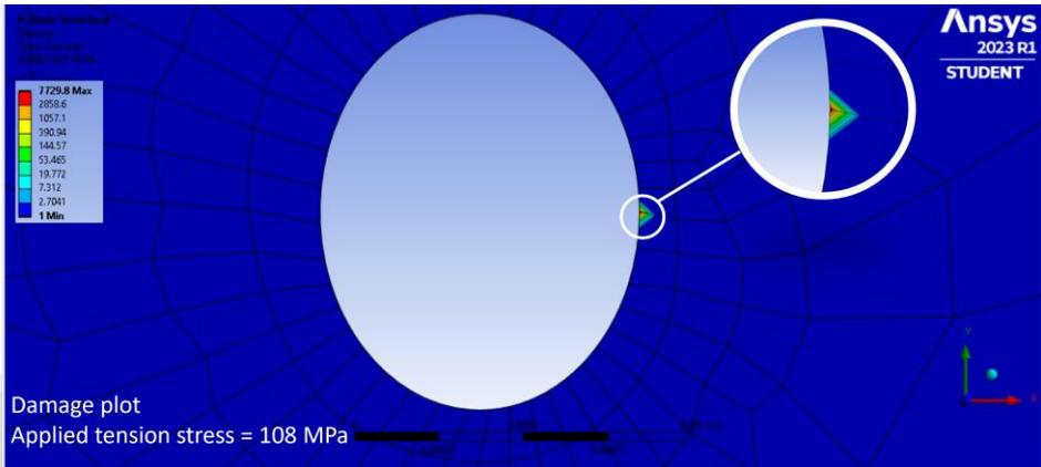
Figure 34: Fatigue Tool Damage plot. Zoom of the circular notch
