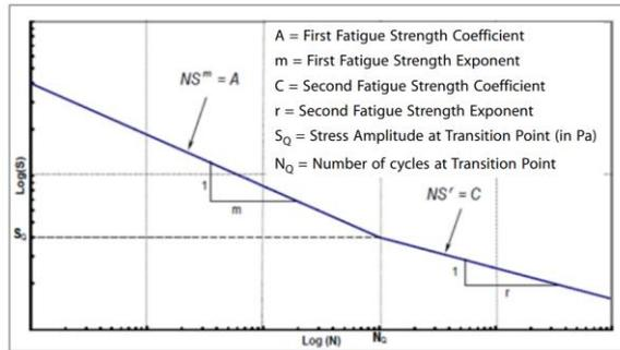
Figure 29. Bilinear S-N curve
