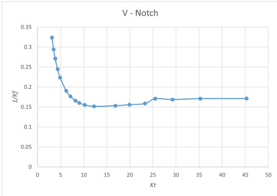
Figure 21: Relation between  $K_f$  and  $K_t$  depending on the radius.
