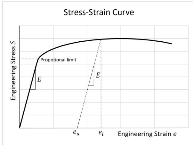
Figure 1: Example of a stress-strain curve obtained with the tensile test.
