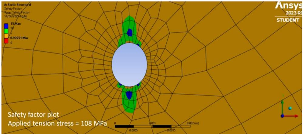
Figure 35: Fatigue Tool Safety Factor plot. Zoom of the circular notch
