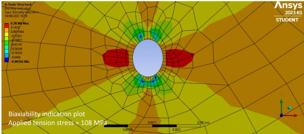
Figure 36: Fatigue Tool Biaxiality Indication plot. Zoom of the circular notch
