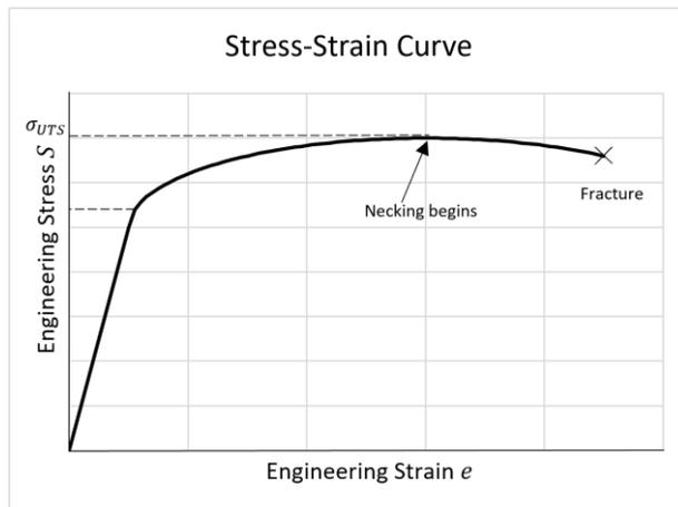
Figure 2: Ultimate tensile strength on the stress-strain curve
