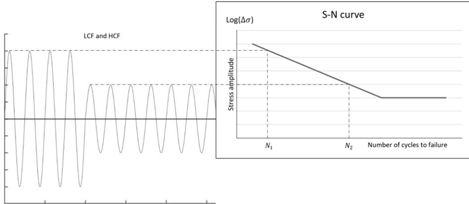
Figure 6: Example of a Wöhler diagram for high and cyclic fatigue
