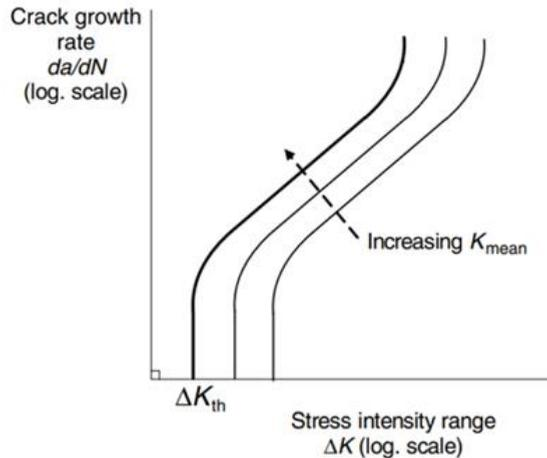
Figure 8: Typical fatigue crack growth rate curves [14]
