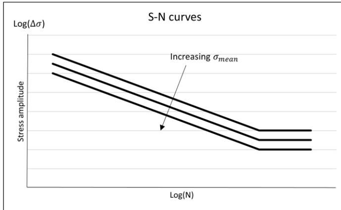
Figure 7: Variation of the S-N curve due to the mean stress
