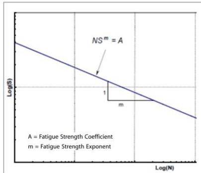
Figure 30. Linear S-N curve
