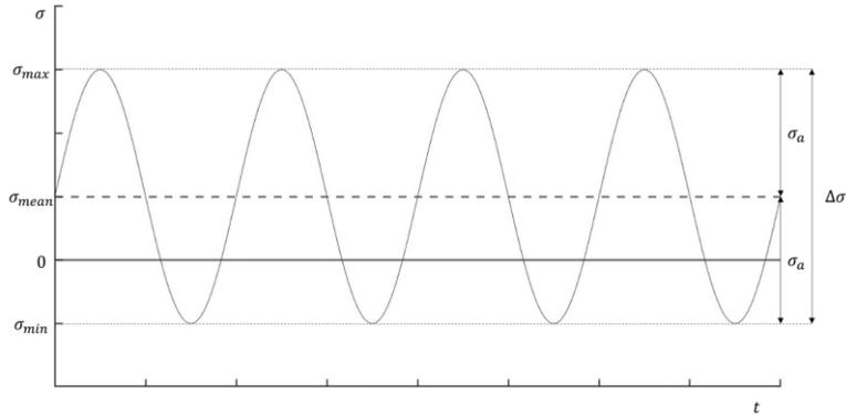
Figure 3: Stress variables for constant amplitude cyclic stress
