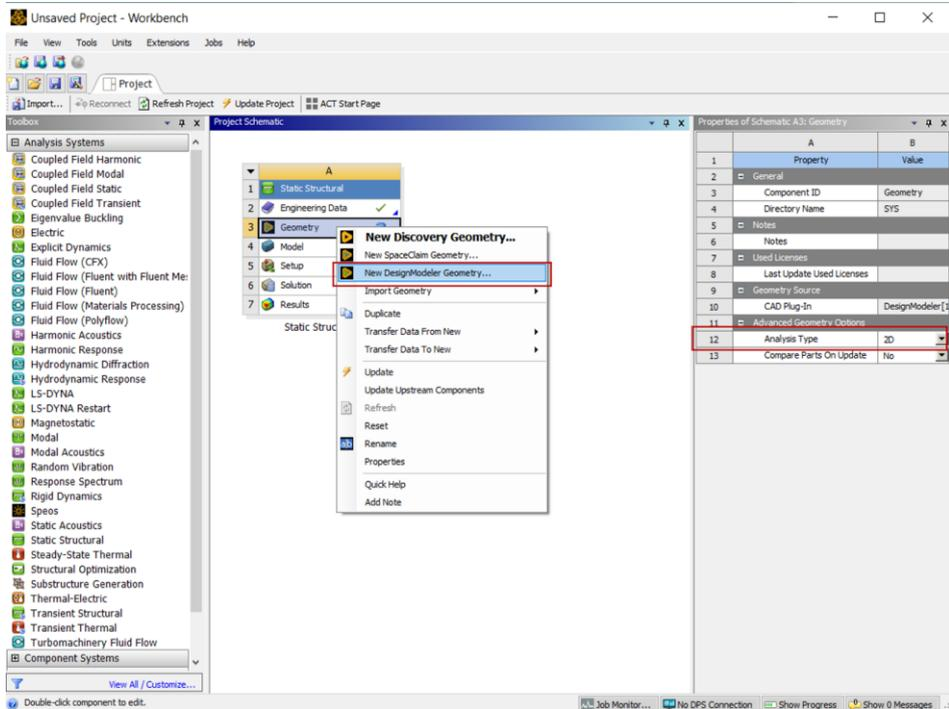
Figure 25: Workbench New DesignModeler Geometry
