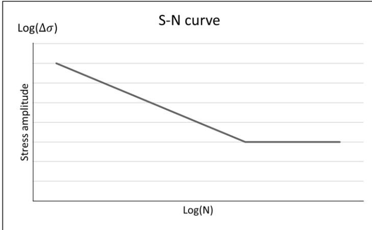
Figure 4: Theoretical S-N curve
