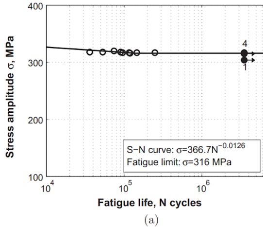
Figure 23: S-N curve of the used stainless steel [3]
