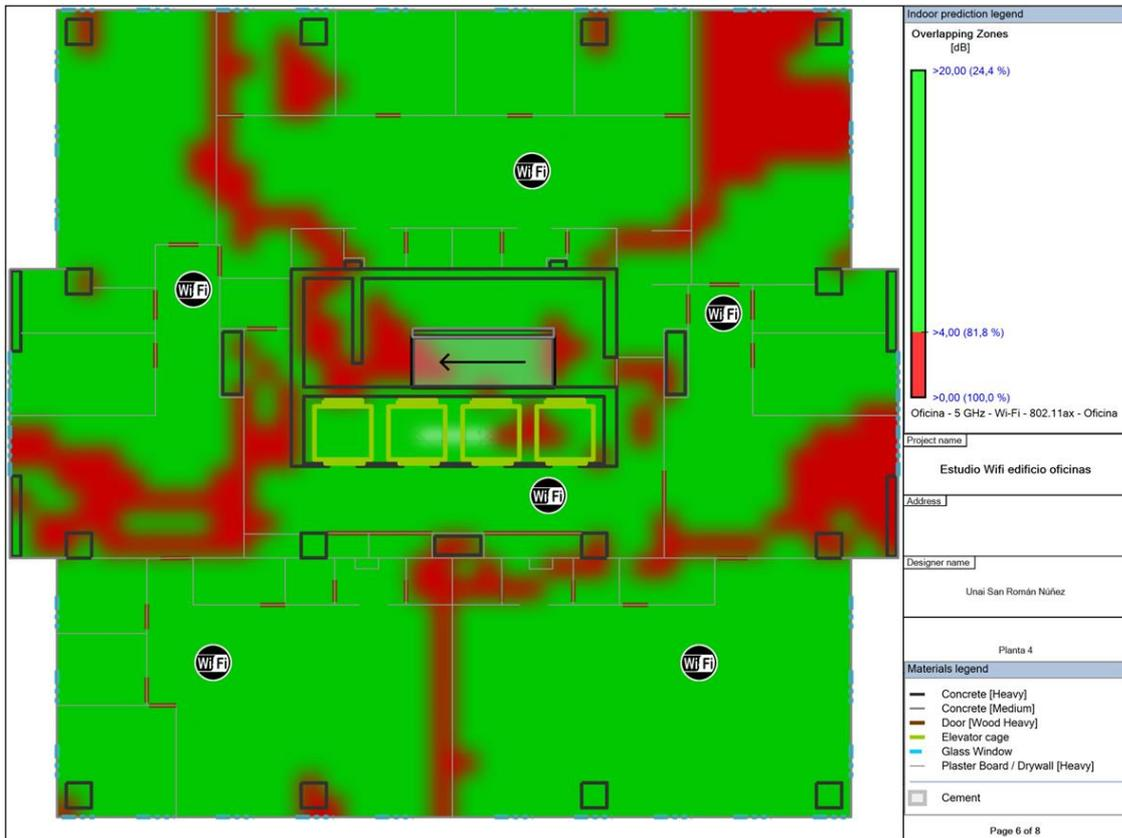
Figura 4-58. Zona de Overlap 5Ghz. Planta 4.
