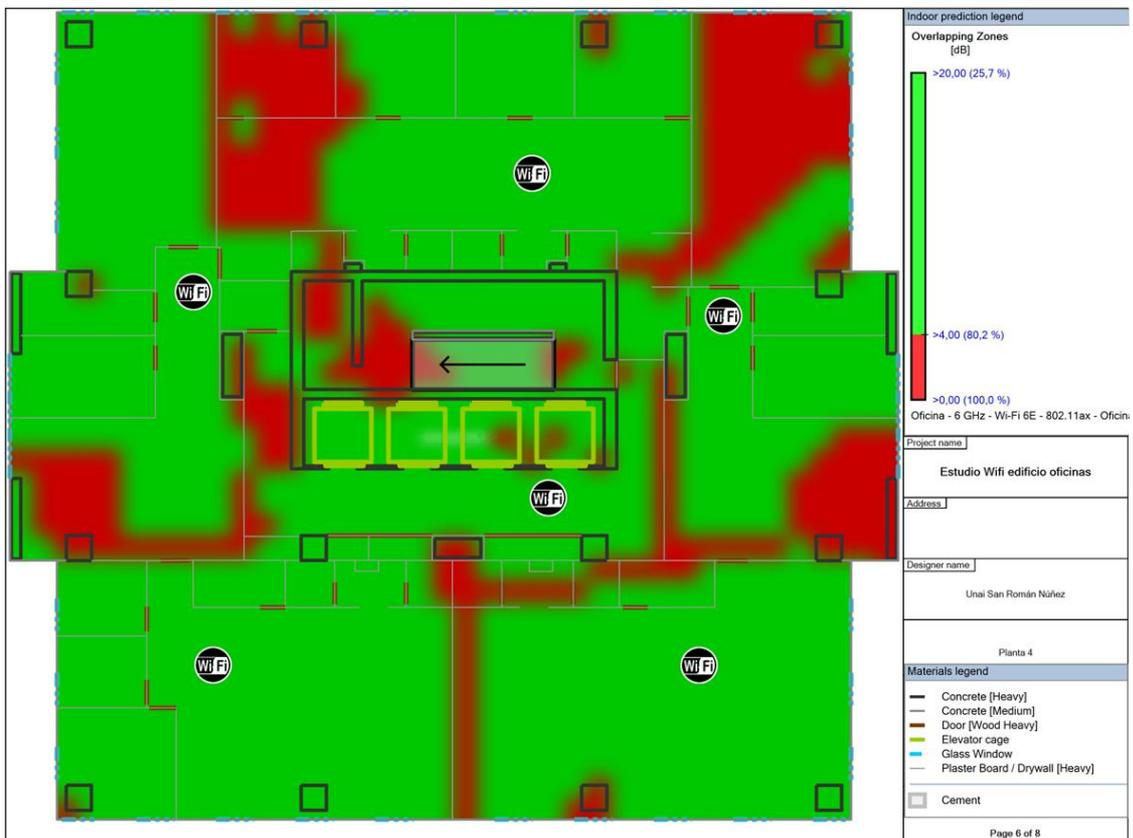
Figura 4-59. Zona de Overlap 6Ghz. Planta 4.
