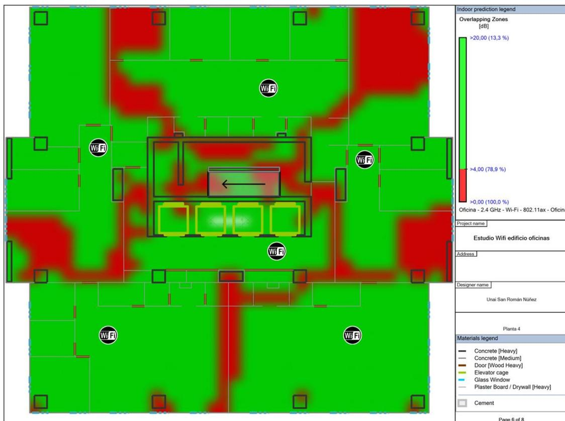
Figura 4-57. Zona de Overlap 2.4Ghz. Planta 4.
