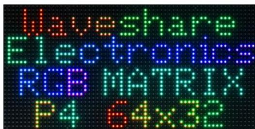
**Figura 3.3** Pantalla LED RGB-Matrix-P4-64x32 [9].
