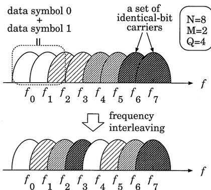
Fig. 8 Frequency interleaving ( $N = 8, M = 2, Q = 4$ ).
