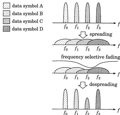
Fig. 2 Power spectrum of an MC-DS-SS signal.
