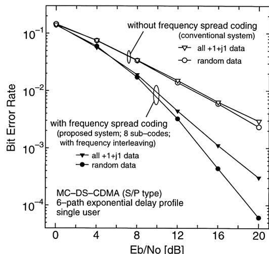
**Fig. 9** Bit error rate performance versus  $E_b/N_0$  for the conventional and proposed MC-DS-CDMA systems; 8 sub-code channels with frequency interleaving (in the proposed system); single user ( $K = 1$ ).
