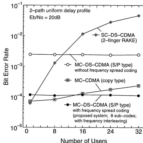
**Fig. 10** Bit error rate performance versus number of users for different CDMA systems;  $E_b/N_0 = 20$ [dB].
