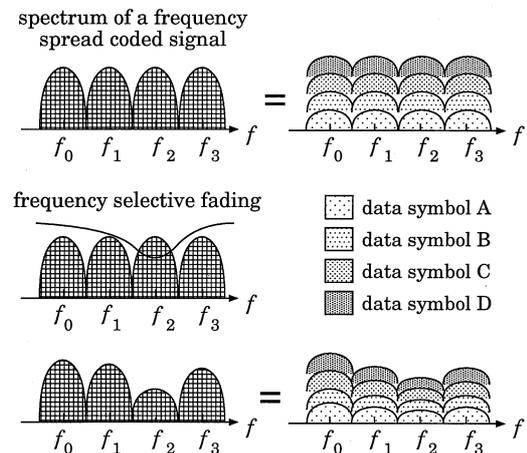
Fig. 4 Power spectrum of a frequency spread coded signal (the same pattern indicates the same data symbol).
