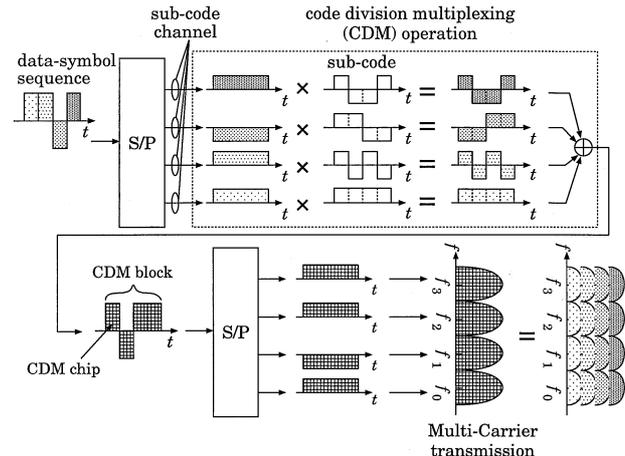
Fig. 3 Principle of frequency spread coding and the power spectrum of the transmitted signal.
