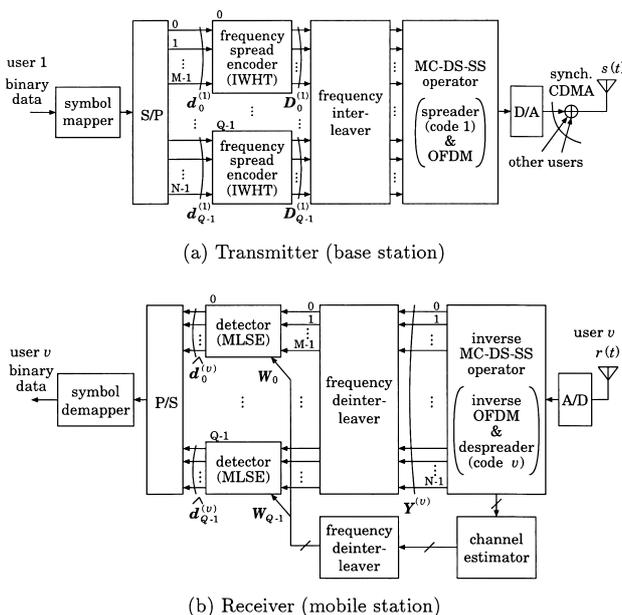
**Fig. 5** MC-DS-CDMA system using frequency spread coding (proposed system).
