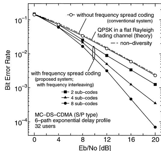
**Fig. 7** Bit error rate performance versus  $E_b/N_0$  for the conventional and proposed MC-DS-CDMA systems; with frequency interleaving (in the proposed system); fully loaded system ( $K = 32$  users).
