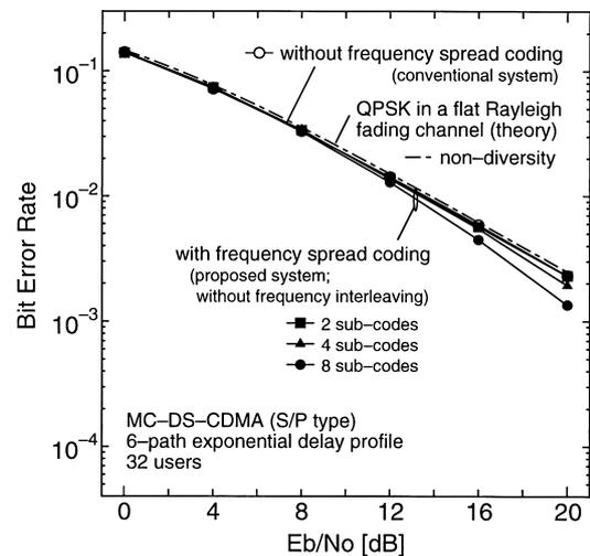
**Fig. 6** Bit error rate performance versus  $E_b/N_0$  for the conventional and proposed MC-DS-CDMA systems; without frequency interleaving (in the proposed system); fully loaded system ( $K = 32$  users).
