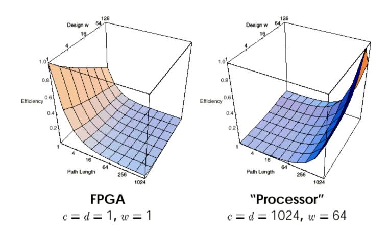
Efficiency comparison between processors and FPGAs (Dehon96)
