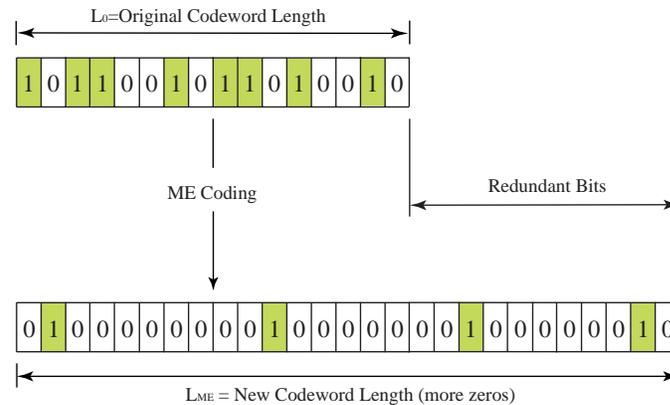
Figure 2.2: *Principle of Minimum Energy Coding.*
