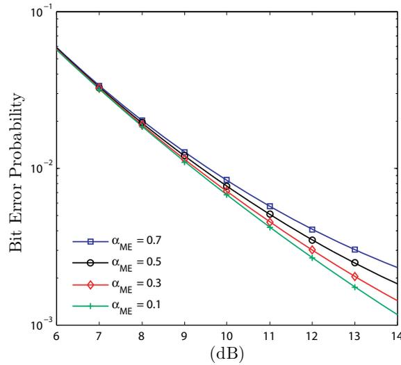
Figure 2.7: *Bit Error Probability with the variation of  $\alpha_{ME}$  in a system using ME Coding when the wireless channel is considered and overall system power is minimized.  $R_b = 250$  Kbps.*
