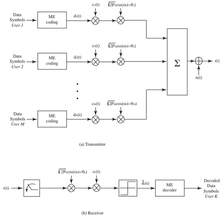
Figure 2.5: DS-CDMA combined with ME source coding.
