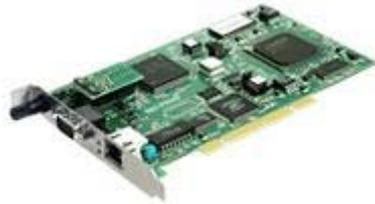
**Figura 15: Tarjeta PCU-2000ETH de Applicom**
