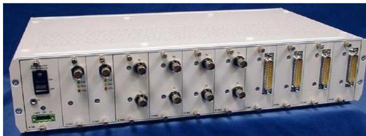
Figura 3.3. Vista trasera nodo Trame+. (Slots 1-4 → KTMV, Slots 5-8 → KTMG, Slots 9 y 10 → KTMX, Slot 11 → KTMi)
